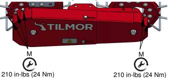
20. Tighten the two 5/16" hex bolts that secure the front and rear covers together. Torque the two bolts to 210 in-lbs (24 Nm).
