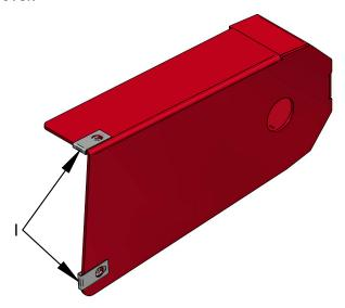
15. Position the front chain cover over the rear chain cover aligning the mounting slots with the U-nut locations (J).
