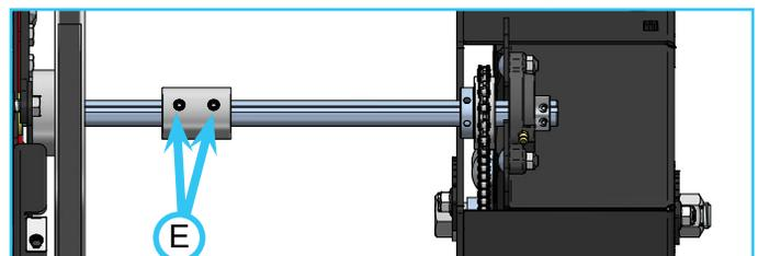
6. Slide the axle shaft coupler onto the half shaft as shown below and remove the key (F).
