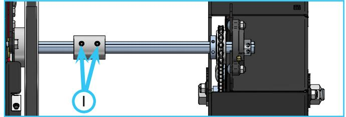
15. Tighten the two set screws (J) in the left outer flange bearing using a 1/8" hex key.
