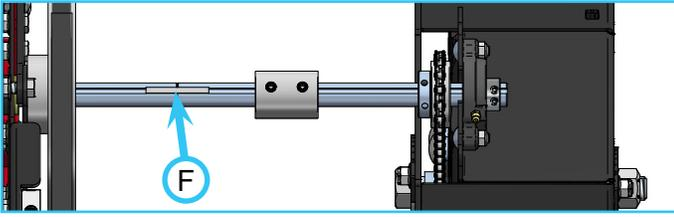
7. Slide the axle half shaft (G) through the flange bearing to allow the belt to pass between the axles.
