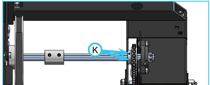
17. Install the sprocket cover. Secure the sprocket cover in place with two 3/8" carriage bolts and locking flange nuts.
