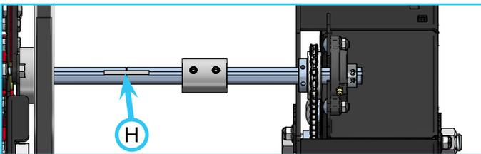
13. Slide the axle shaft coupler over both axles aligning the set screws with the key.
