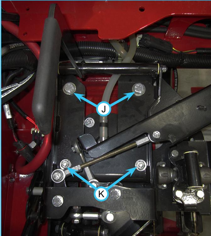
15. Remove the two 3/8" bolts (K) from the shifter mounting bracket.
