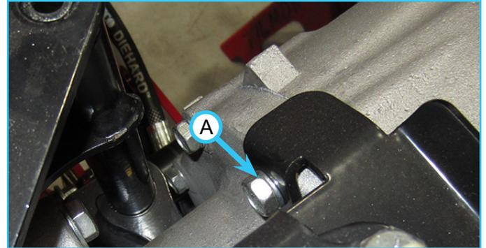
3. Torque the two 8mm bolts to 22 ft-lbs (30 Nm).
