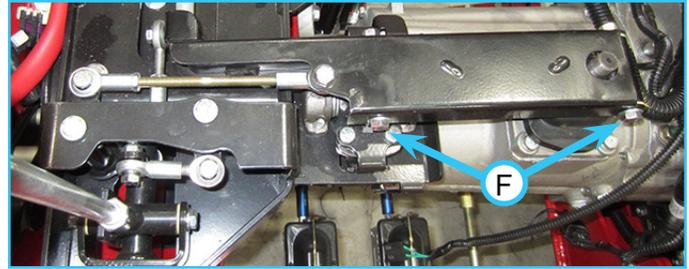
13. Torque the 5/16" bolts to 210 in-lbs (24 Nm).
