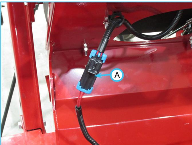
2. Disconnect the operator presence sensor.
