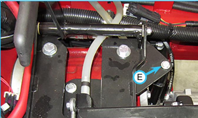
11. Torque the 5/16" bolt to 210 in-lbs (24 Nm).
