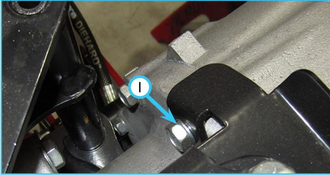
14. Remove the two 1/2" bolts (J) from the shifter mounting bracket.
