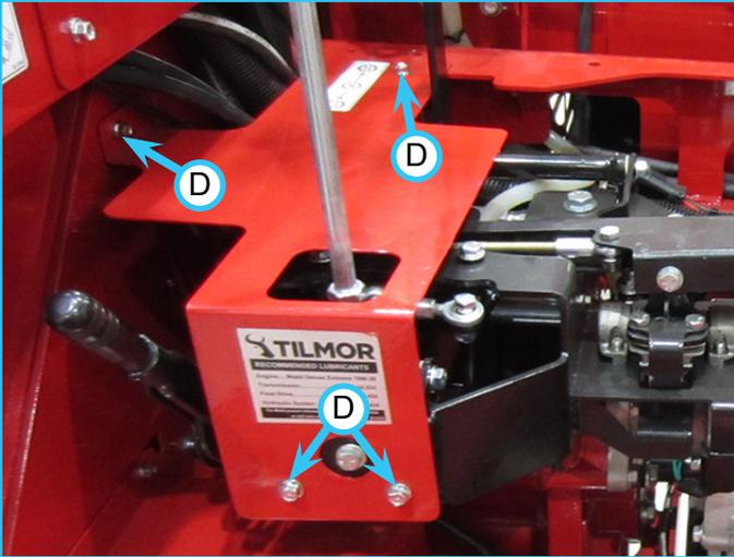
8. The shifter box cover can now be lifted over the shifter handle and removed.
