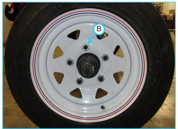
10. Torque the lug nuts to 100 ft-lbs (135 Nm), alternating between the bolts in a alternating pattern to ensure the wheel is tightened to the hub evenly.
