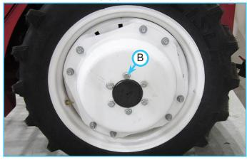
9. Torque the 9/16" wheel stud bolts 130 ft-lbs (176 Nm).
