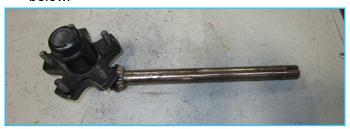
13. Install the new spindle assembly into the bottom of the axle pivot tube, aligning the keyway (F).
