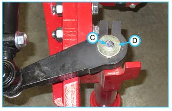
8. The spindle assembly can now be removed from the bottom of the axle pivot tube.
