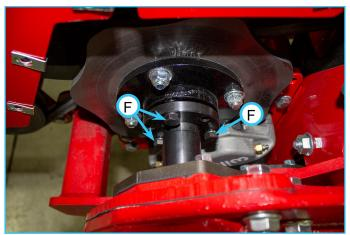
12. Install two of the bolts (G) into the threaded holes. Using rotating quarter turns between the two bolts to remove the hub from the rotor.
