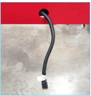
4. Remove the caps from the wiring harness.
