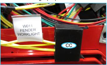
59. Connect the rear work light connector (BB) to the rear work light rocker switch and the fender work light (CC) to connector to the fender light rocker switch.
