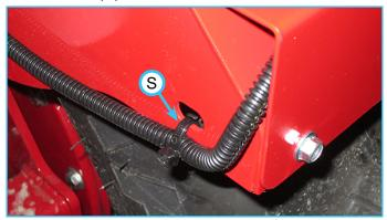
31. Secure the two branches of the harness to the main wiring harness using a cable tie as shown below.
