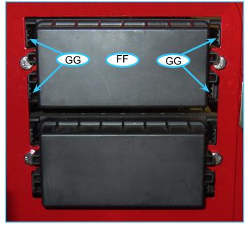
65. Reference the fuse block diagram, located on the inside of the fuse panel access door for the installation location of the two 10 amp mini fuses.
