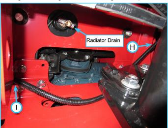
10. The long side of the harness will be routed under the engine radiator and through opening (I).
