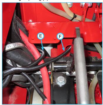
8. Pull the short side of the harness (G) through the opening above the hydraulic filter located at the rear of the tractor between the engine compartment and the right fender assembly.
