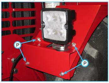
25. Torque the bolts to 100 in-lbs (11 Nm).
