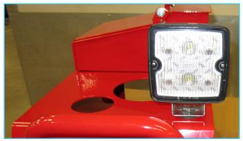
45. Secure the light in place with the 3/8" washer and 3/8" lock nut on the inside of the fuel tank cover.
