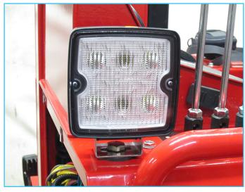
35. Secure the light in place with the 3/8" washer and 3/8" locknut on the inside of the operators console.
