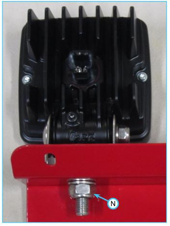
16. To install the left rear work light mounting bracket, route the harness through the work light mounting bracket.
