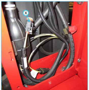
48. Route the harness through the access panel over the fuel tank in line with the fuel lines.
