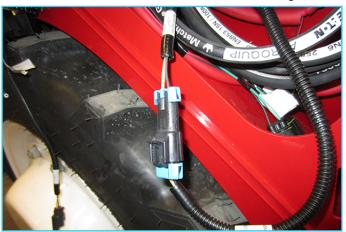
34. Install the right front work light, position the 3/8" mounting bolt through the rubber washer, and then through the console.
