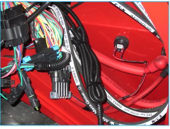
33. Connect the wiring harness to the tractor wiring harness connector labeled Rear Work Light.
