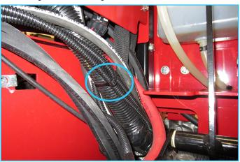
32. Bundle the harness together with two cable ties inside the operators console.
