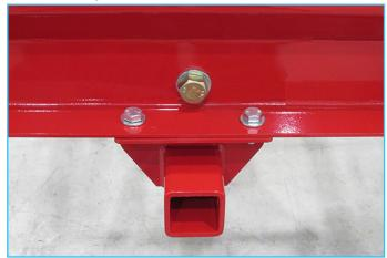
3. Align the mounting holes (B) under the front axle.
