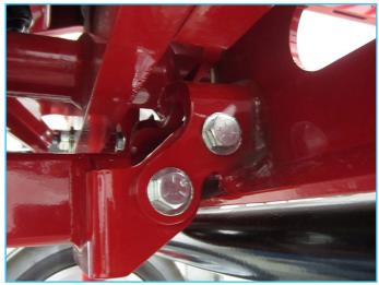
5. Tighten the bolts in an alternating pattern ensuring that the edge of the hitch weldment is flush with the front frame (C) as shown below.
