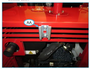
71. Secure the bracket in place using two 1/4" flange bolts and two 1/4" flange nuts.
