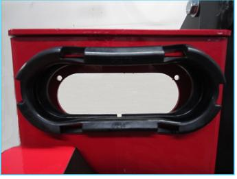
45. Install the six light adapter harnesses onto the six lights. Ensure that the harness connections are fully seated on the lights.
