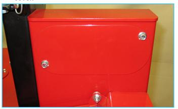
43. Remove the left and right rear marker light covers by removing the four 1/4" bolts from each cover.
