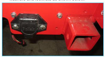
54. Torque the 1/4" bolts to 100 in-lbs (11 Nm).
