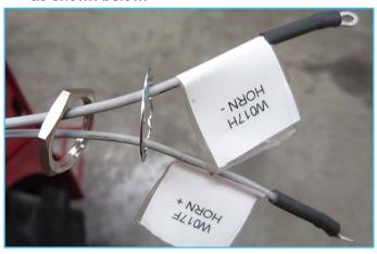
11. Route the horn wires over the hydraulic valve and through the horn switch mounting hole.
