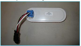
46. Install the forward facing left and right amber marker lights into the grommet. Firm pressure is required to fully seat the light in the grommet.
