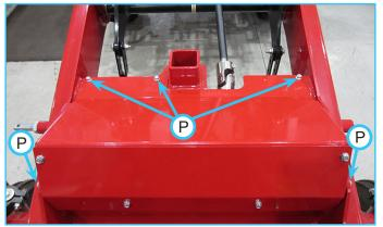
21. Torque the 1/4" bolts to 100 in-lbs (11 Nm).
