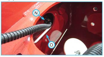
Route the harness through the frame to the harness access hole located under the front hitch hydraulic cylinder.
