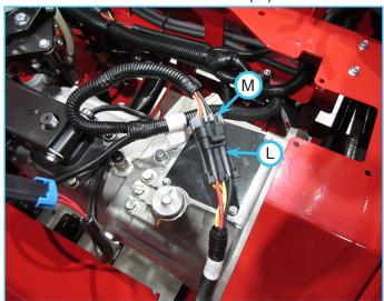
15. Bundle the wiring harnesses together neatly on top of the transmission and secure in place with cable ties.
