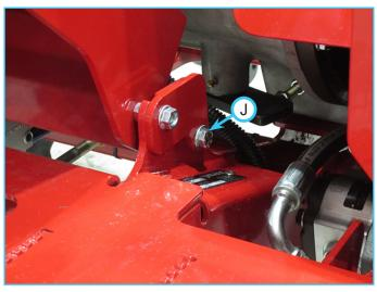
11. Install the cushioned clamp over the wiring harness.
