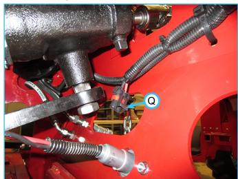
30. Connect the front harness to the 12 volt plug connector as shown below.
