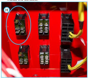
13. Connect the W016 12V Aux Front connector to the rocker switch as shown below.
