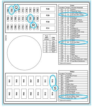
26. Install the 15 amp mini fuse in terminal F04 (12V Aux R11 / R13) and the 30 amp mini fuse in terminal F20 (12V Aux Rear) in the upper fuse block.
