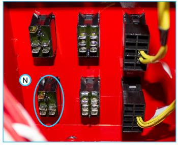
19. Connect the W016 12V Aux Rear connector to the rocker switch as shown below.
