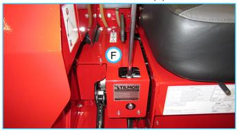
11. Locate the wiring harness labeled Rear Harness 12V Aux behind the 2-speed shifter (G).
