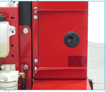
24. Remove the upper and lower fuse block covers by squeezing the four black plastic tabs (P) toward the cover, and pulling the cover off.
