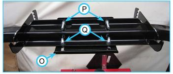
25. Attach the L-Clamp bracket to the roll bar bracket using two 3/8" x 1-1/4" bolts and lock nuts (Q) to bottom front mounting location.
