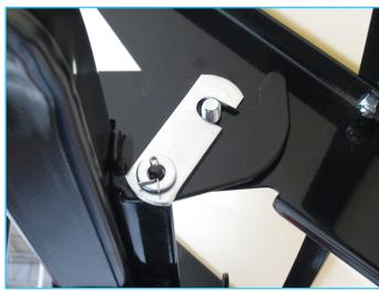
31. Attach the clamp knobs (R) to the mounting bolts on both sides of the TuffTop and tighten the knobs to secure the TuffTop in place.
