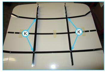
Secure each strut in place using two 1/4" x 3/4" bolt and lock nut (K).
