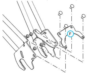
Tighten the handle bar cross plate and the connector plate alternating between all of the bolts. Frequently check the operation of the drive control handles ensure that the handles move freely with no binding.
