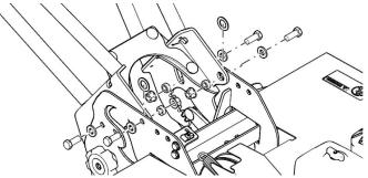
9. Route the drive control cable (G) through the handle bar frame at points (H).
