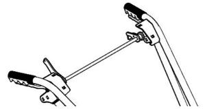
4. Install the handlebar cross plate (E). Secure the plate in place using four 5/16 x 3/4" carriage bolts and locknuts tightened hand tight.
