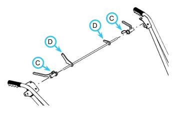
3. Install the handlebar frames onto the pivot shaft.
