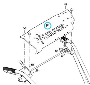
5. Install the handle connector plate (F). Secure the plate in place using four 3/8 x 1" carriage bolts and locknuts tightened hand tight.
