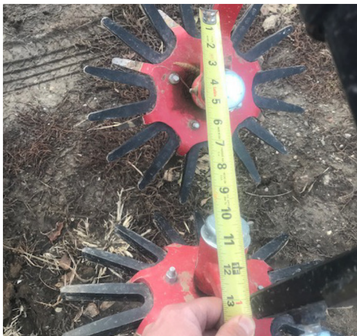
fig. 10: measuring the distance between finger-weeders
