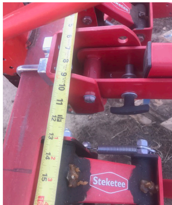
fig. 7: marking the rows on the toolbar.
