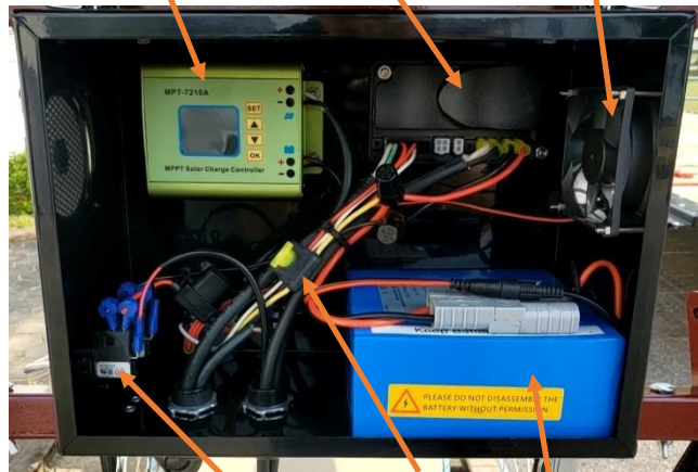
steering switches | 5A fuse | battery
