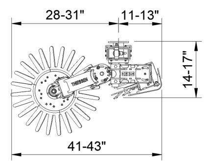
Overall length of the unit is 41" as shown above, but can extend to 43" when the finger weeder head flexes towards the tractor
