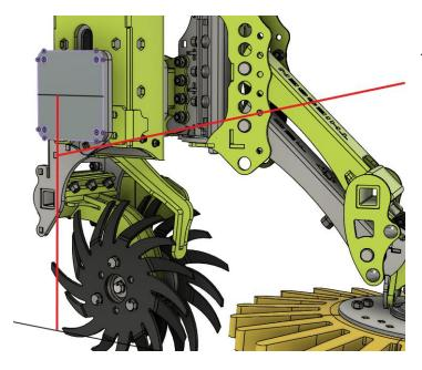
The centre line of the mating plate on the tractor should be a 10-16" above ground level.
