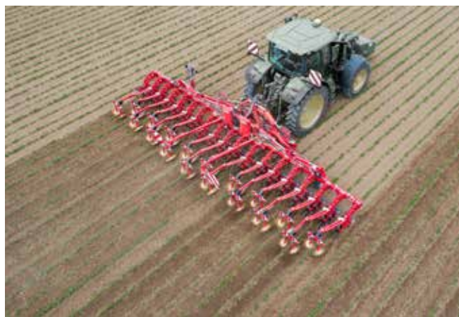
Rear hoeing with camera steering and double folding frame
