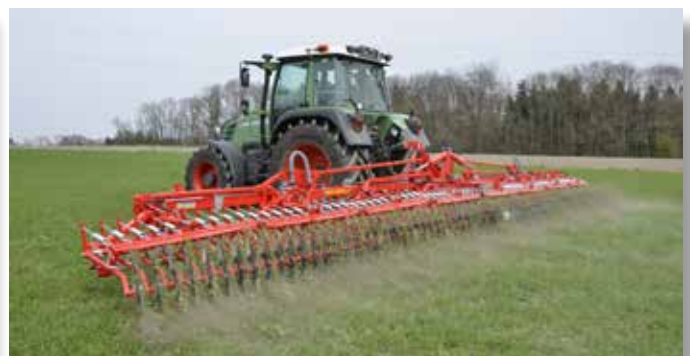
Weeding in spring using a rotative weeder
