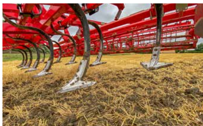
Duckfoot sweeps mounted on spring tines
