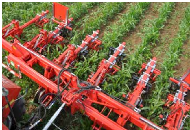
Rotative row-crop cultivator with rear upper link steering
