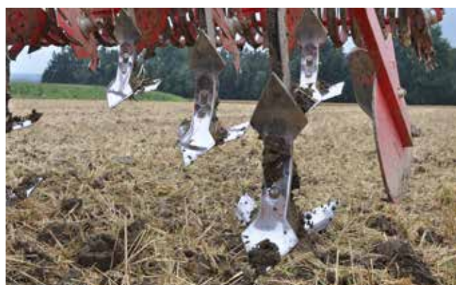
Sweeps mounted on rigid shafts in addition to double-heart sweeps
