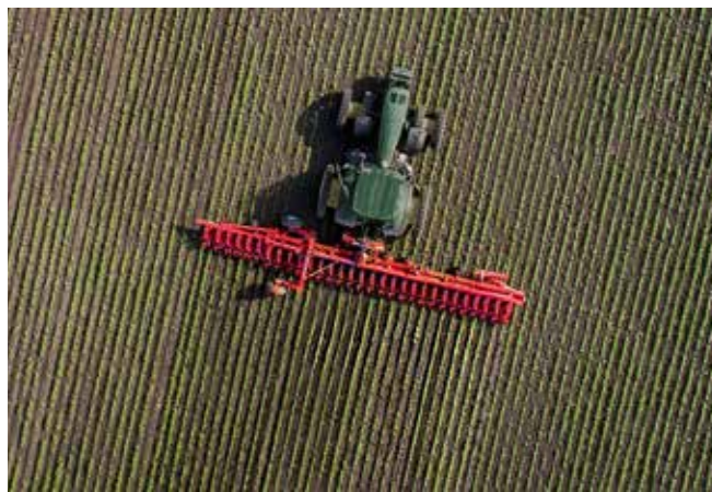
Rear hoeing with camera steering and longitudinal drive unit
