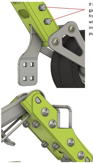
If you are using the offset shank directly behind the gauge wheel for an A-blade then next use the hardware from the RED bag to secure it in place. The flange nuts will be slipped into the hex shaped holes from the inside and then the bolts can be threaded through and pushed up against the shank to secure it in place.
