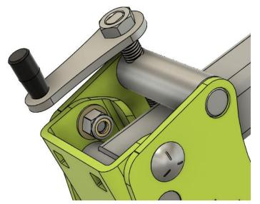
Next install the gauge wheel height adjust handle. It may require gentle tapping to get it into place on the threaded shaft, and then can be secured with the thin 12mm nut. To tighten the nut, hold the hand secure and snug the nut with a wrench or ratchet and socket.
