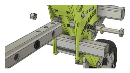
The parallels are designed to accept an 18 or 24" modbar in the back that can pivot like a trailing arm to give tooling some independent float vs the fixed tooling mounted directly to it. The trailing modbar can also be clamped solid if float isn't desired. Hardware for this application is in the YELLOW bag.
