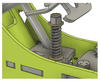
If using the pivoting modbar, then use the 4" carriage bolt and install it with two washers, a nylock nut and one of the springs as shown to the left. It may be a bit easier to insert the bolt if you tip the modbar up a bit at the back and temporarily remove the lower 250mm modbar.
