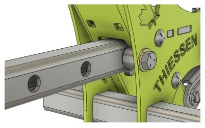
Install the modbar so that the three smaller holes are at the end closer to the body, with the square holes facing down. Insert the plastic bushings into the second set of 16mm holes.
