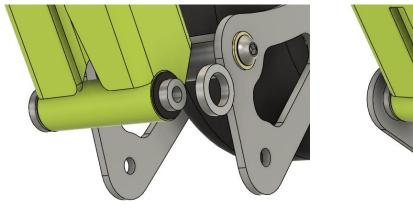
The first step is to install the gauge wheel pivot pin into the bottom of the main body using the hardware found in the BLUE bag. The axle will first slip into the plastic bushings pressed into the body with the two thick washers slipped over the ends. The gauge wheel arms can then be swung over and bolted down with the two button head cap screws and washers.
