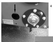
Pressure wash the conveyor rollers weekly through the four round holes to insure longer life of the conveyor belt.
