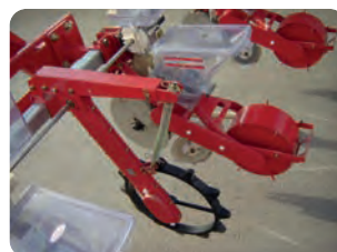
PELLET DISTRIBUTOR DRIVE SYSTEM (JPH OPTION)
