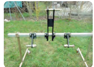
CAT. 2 TRACTOR 3-POINT HITCH - WITHOUT BAR (JPH / JTS-600/1200 OPTION)
