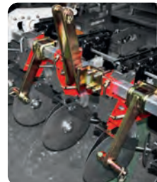
CAT. 1 MICROTRACTOR HITCH (WITHOUT BAR) (JPH / JTS-600 OPTION)
