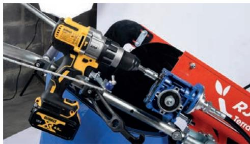
(23) Fit the drill onto the arm of the machine by pushing the chuck onto the hexagonal shaft.
