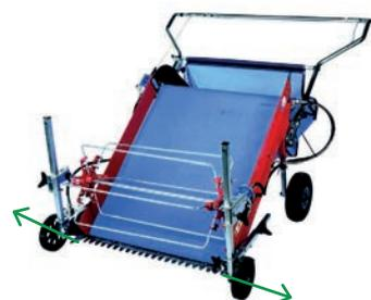
(15) Insert the horizontal tube of the wheel in the front tube of the machine: the star screw must face the inside of the machine and the wheel must be on the outside.
