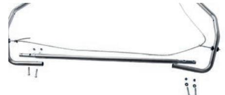
(9) Connect the central bar to the left and right arms of the push bar.
