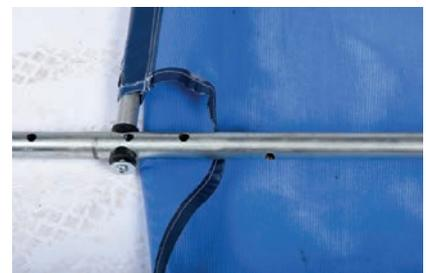
(12) Thread the assembly into the holes in the frame and put the bolts through the holes, when they are aligned.
