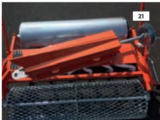
As it turns, the seed reserve will loosen the chain no.20. Remove the chain from the sprocket no.21 and recover the seed reserve.
