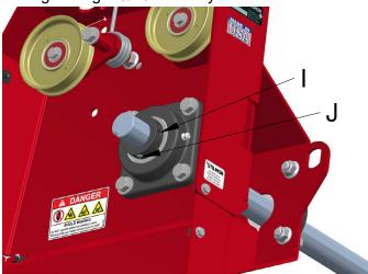
Using a punch and hammer loosen the collars by placing the punch in the indent (I) and hitting the collar.
