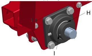
Using a punch and hammer loosen the collars by placing the punch in the indent (I) and hitting the collar.
