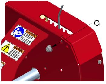
7. Position the new tensioner in the top cover inserting the mounting bolt through the upper mounting hole (H).
