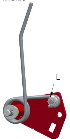
12. Position the new tensioner in the top cover. Insert the tensioner mounting bolt through the upper mounting hole (M).
