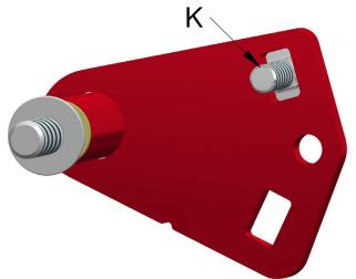
10. Position the new torsion spring on to the mounting bracket. 11. Secure the torsion spring in place using a 3/8" locking flange nut (L). Torque the flange nut to 31 ft-lbs (42 Nm).
