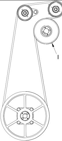
13. Set the belt tension as required by adjusting the tension adjustment lever.
