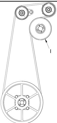
14. Reinstall the pulley cover. Torque the 1/4" bolts to 100 in-lbs (11 Nm).
