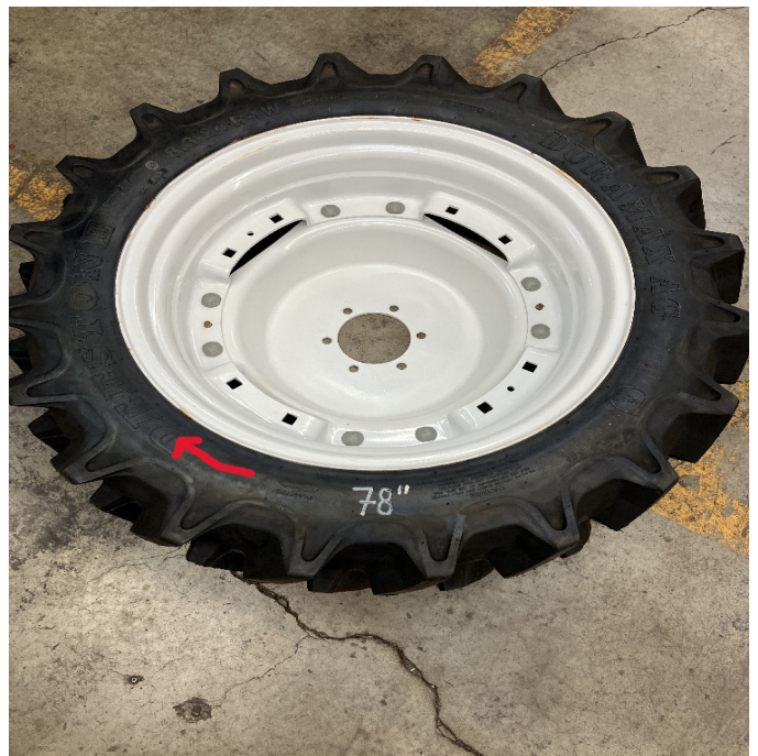
Right side wheel oriented for 78" spacing. Note: for 78" spacing, entire dish, rim and tire assembly can be swapped from one side to the other without any disassembly (when starting with 50" standard spacing).
